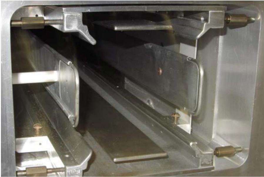
Figure 3.3: Photograph of one ESQ station. For vertical confinement of (positive) muons, the top and bottom plates are positively charged whereas the lateral plates are charged with negative voltage. The vertical magnetic field in the storage ring largely contributes to stable motion in the horizontal direction, in spite of the defocusing radial gradient from the ESQ inner and outer plates.
