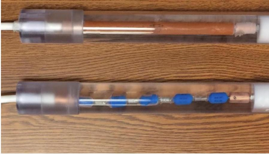
Figure 3.62: Single-CADDOCK high-voltage resistor (top) and chain of potted HV resistors (bottom). Two of the latter type of resistors became damaged during Run-1.
