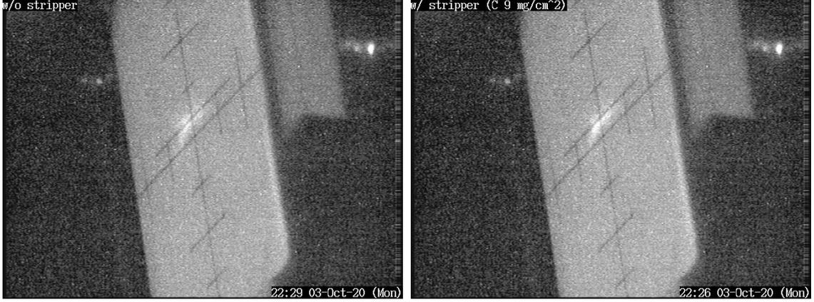
Figure 3.10: Beam spot on a ZnS scintillation target at the target position with (right panel) and without the stripper foil (left panel). Ticks on the target are marked in 5 mm step.
