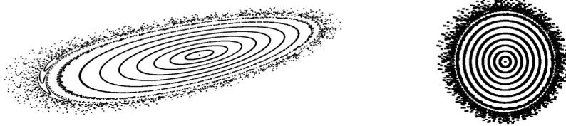
**Figure 1.1:** *Phase space trajectories in FODO cell, obtained for 1000 turns by applying one turn map to the vector with initial coordinates 1000 times; in conventional (left) and normal form (right) coordinates*
