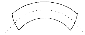
Fig. 1. A magnetic sector with tilted and curved effective field boundaries. The dashed line is the reference orbit.
