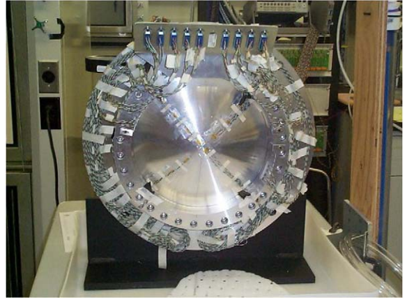
Fig. 1. Example of a torospherical window for sFOFO-type absorber in testing phase.
