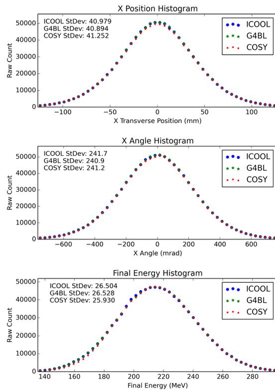
Figure 3: MICE Step IV  $x$  position,  $x$  angle, and final total energy results for 65 mm of lithium hydride.
