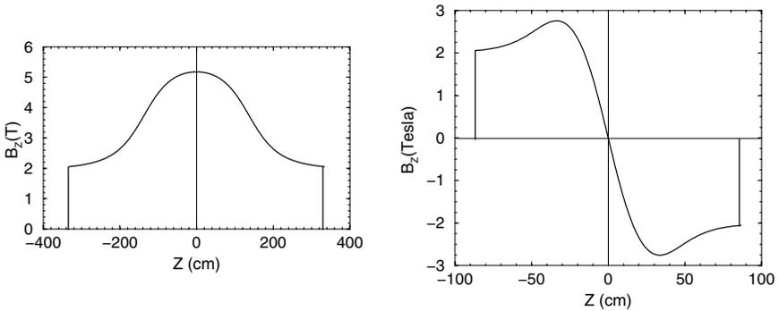
Figure 4. The hard edge model of the axial magnetic field in the long straight solenoidal section (left) and in the short straight solenoidal section (right), assuming the solenoid coils extend to infinity[1].
