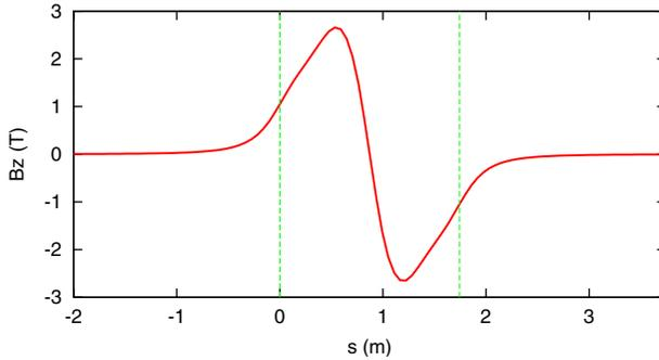
**Figure 5.** The axial magnetic field profile of the short section with finitely long solenoids and fringe fields.
