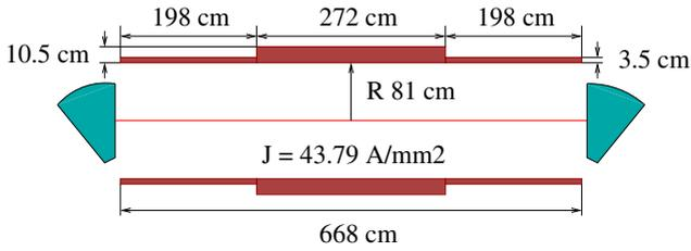
Figure 2. The parameters of the long straight solenoidal section[1].
