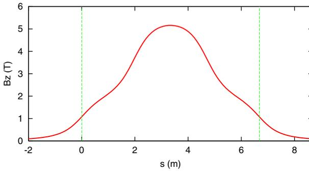
**Figure 6.** The axial magnetic field profile of the long section with finitely long solenoids and fringe fields.
