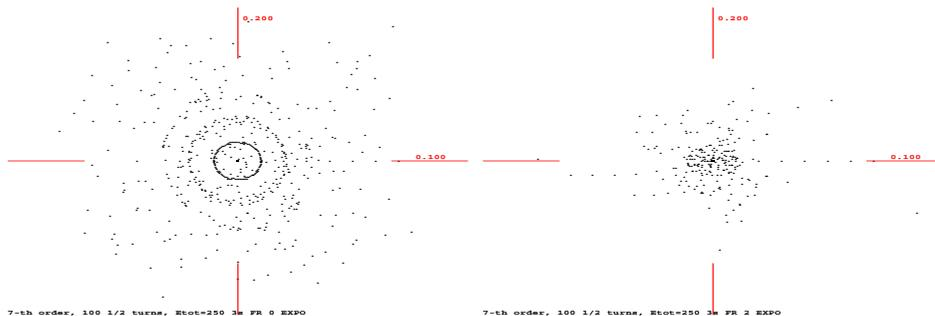
**Figure 9.** Tracking 50 revolutions at reference energy of  $E_{tot} = 250$  MeV with finitely long solenoids with correct fringe field consideration, using hard edge dipole fields (left) and realistic dipole fringe fields (right).
