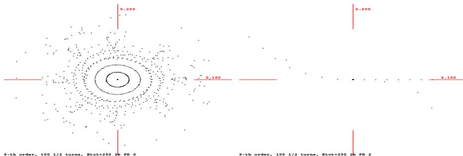
**Figure 8.** Tracking 50 revolutions at reference energy of  $E_{tot} = 250$  MeV with finitely long solenoids in hard edge kick approximation, using hard edge dipole fields (left) and realistic dipole fringe fields (right).
