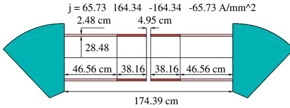
Figure 3. The parameters of the short straight solenoidal section[1].
