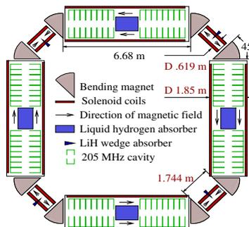
**Figure 1.** The layout of the tetra muon cooler designed by V. Balbekov[1].
