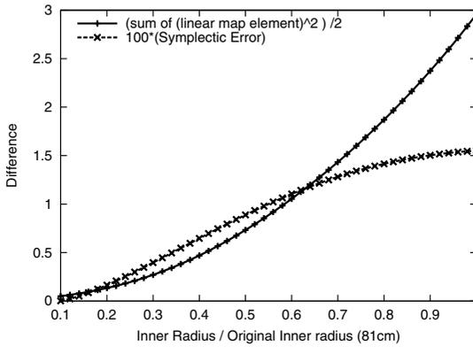
**Figure 7.** The disagreement of the linear transfer maps between the hard edge model and the correct fringe field treatment for the finitely long solenoids of the long section as functions of the aperture.
