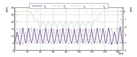
Fig. 2. Optics functions at a three-fold symmetric section of the delivery ring (DR) where the longitudinal distance of the beamline is shown in the horizontal axis. Fringe fields modeled in simulations change the beta functions,  $\beta_x$  and  $\beta_y$ , by less than 3%. Optics functions have served as a channel to validate our BDS model.
