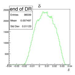
Fig. 4. Beam relative momentum distribution at the storage ring entrance from simulations. One of the main goals of the beam delivery system is to maximize the number of muons with momentum offsets  $|\delta| < 0.5\%$  that are within the momentum acceptance of the storage ring.
