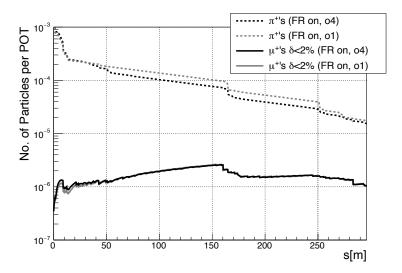
Fig. 5. Simulation results of the number of pions and muons with  $|\delta| < 2\%$  per POT under up to 4th order (o4) effects along the M2/M3 lines with fringe fields (FR) turned on. The longitudinal distance along the M2/M3 lines is shown in the horizontal axis. As depicted by the overlapping curves of the muons population for the two o1/o4 cases, linear simulations do not significantly differ from results when high-order terms in the computation of the particle dynamics are simulated.
