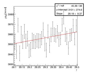
Fig. 9. Beam average of the spin projection angle in the horizontal plane with respect to the reference optical axis,  $\langle \varphi_a \rangle$ , versus the Lorentz factor,  $\gamma$ , at the exit of the delivery ring after four turns. Simulation results presented in this figure correspond to our COSY-based BDS model with fringe fields turned on.
