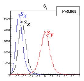
Fig. 7. Histogram of the normalized muon beam spin components (in natural units) at the storage ring entrance from the COSY-based BDS model simulations. The high polarization, P, of the beam is centered with the horizontal plane.
