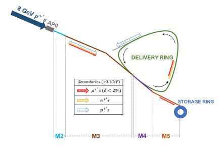
Fig. 1. A schematic layout of the beam delivery system (BDS). Secondary particles (mostly pions, muons, and protons) downstream the target station at APO are canalized through the M2/M3 lines and injected to the Delivery Ring (DR) where protons are discarded after four turns. A cleaner beam of mostly muons is extracted to the M4/M5 lines and ultimately delivered to the Muon g-2 Storage Ring (SR).
