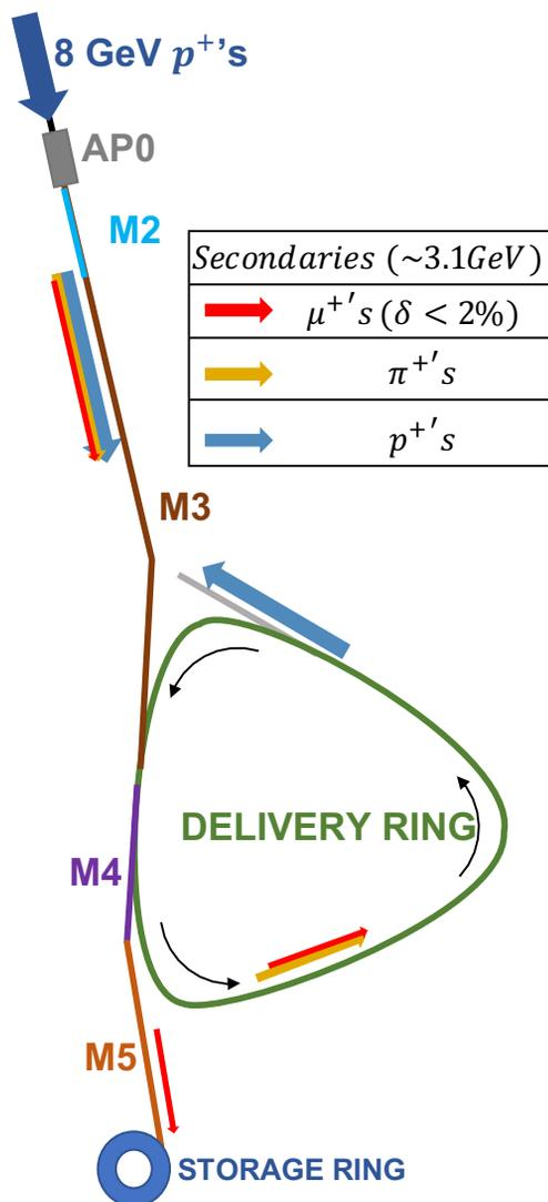
Figure 1: A schematic layout of the BDS.
