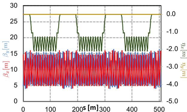
Figure 2: DR optics functions. Fringe fields considered in simulations change the beta functions by less than 3%. The dispersion horizontal function ( $\eta_x$ ) reveals the three-fold symmetry of the ring. Optics functions have served as a channel to validate our BDS model.
