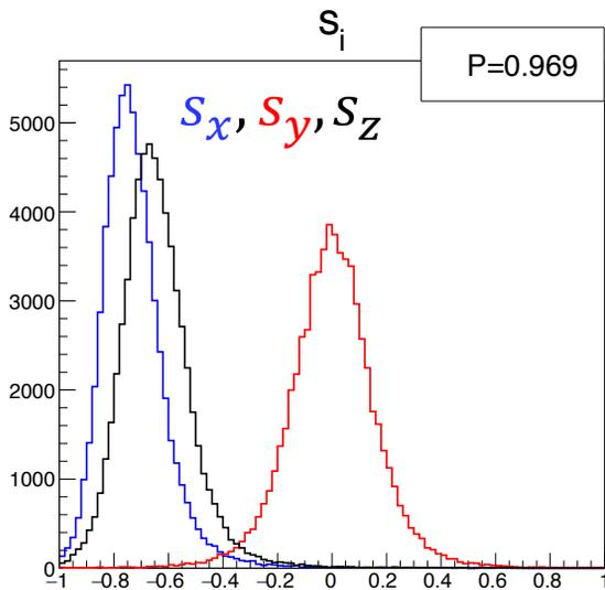
Figure 6: Muon beam spin components at SR entrance.
