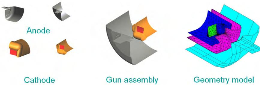
Fig. 9. Parts, assembly and geometry model of a sheet-beam gun.
