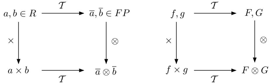
Figure 1: Analogy between the floating point representation of real numbers in a computer environment (left figure) and the introduction of the algebra of Taylor polynomials in the differential algebraic framework (right figure).
