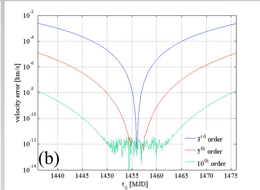
Errors on position, (a), and velocity, (b), between the DA and the point-wise evaluation of Mars ephemerides
