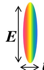
**Bunch compression reduces bunch length and increases energy spread**
