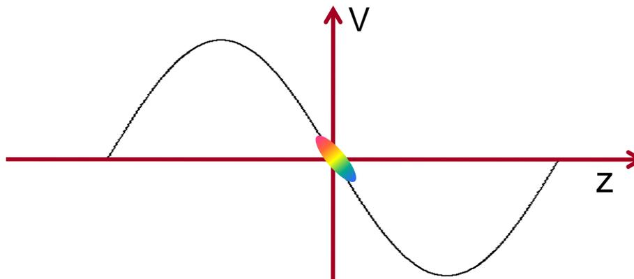
**Phase jitter leads to energy and timing jitter**
