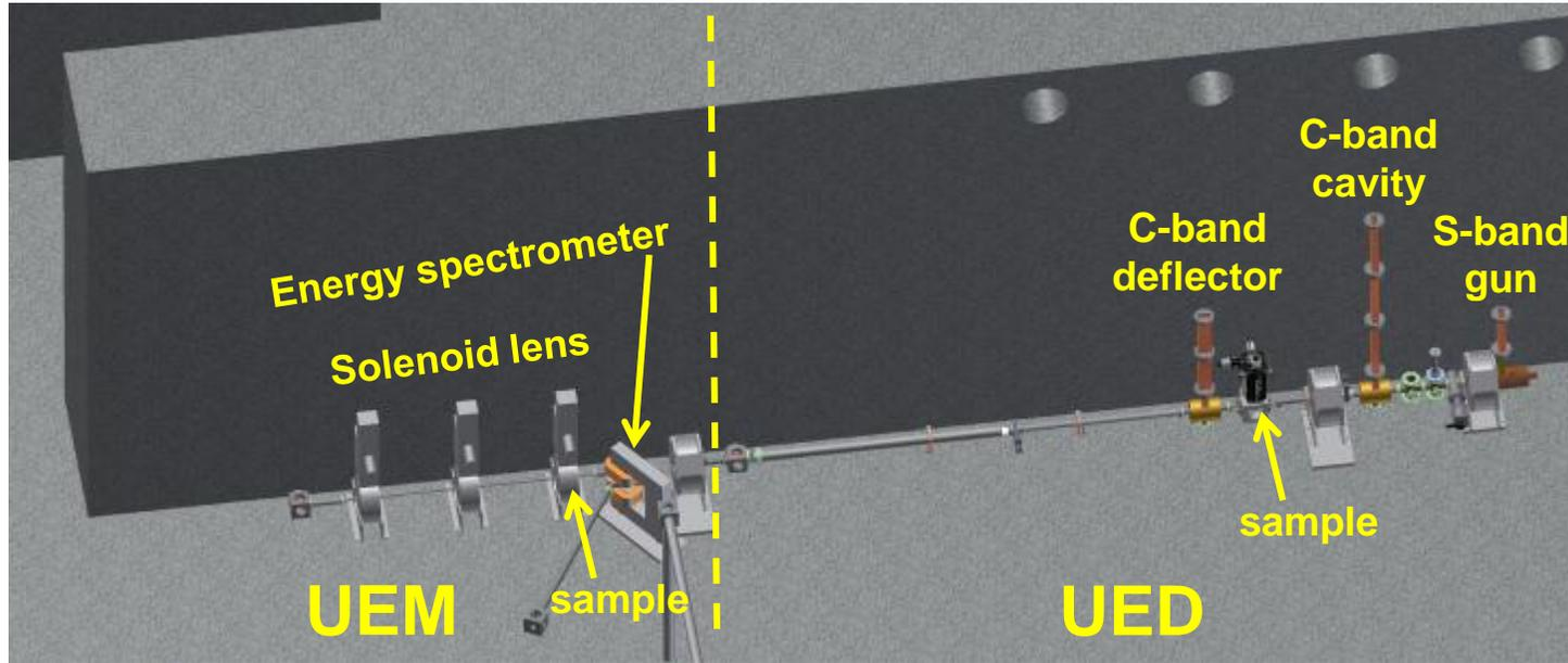
C-band cavity used to remove beam quadratic energy chirp
