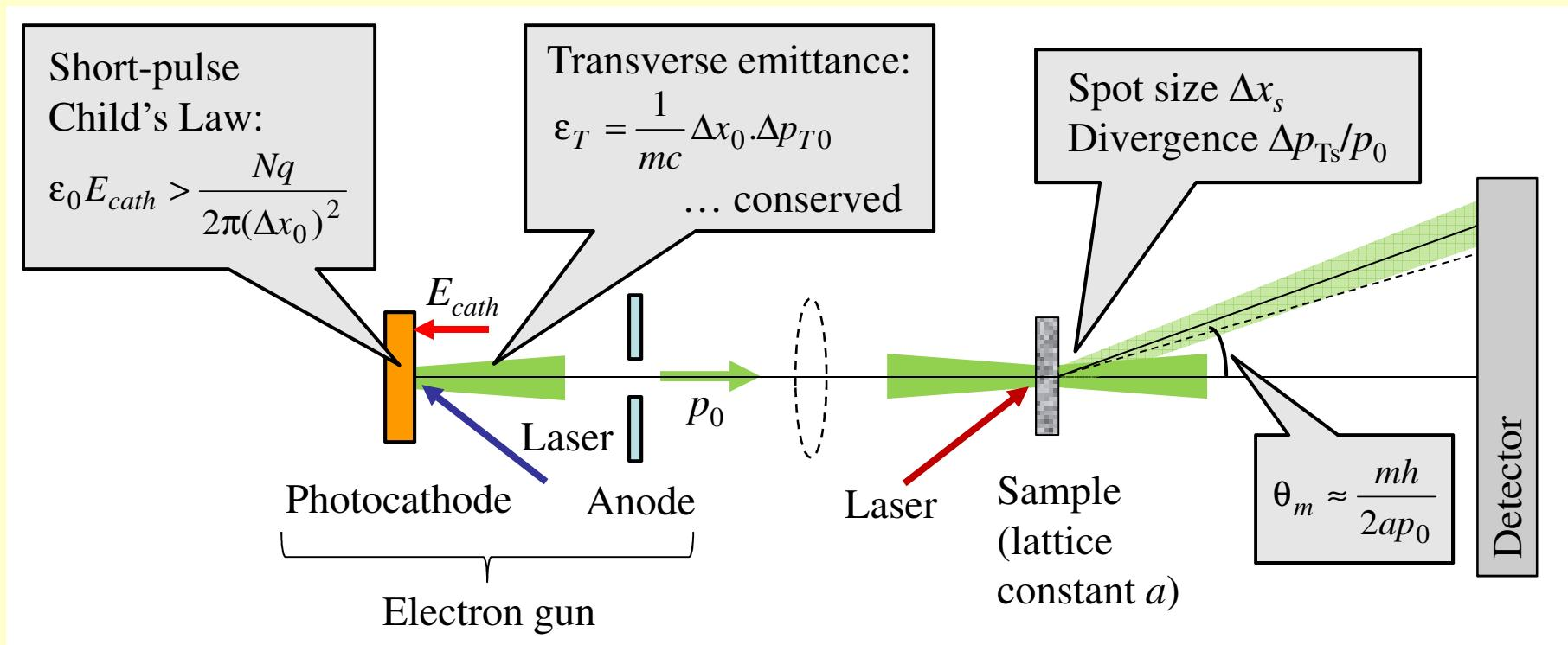
$$\Rightarrow \text{Observable } \frac{\delta a}{a} \geq \frac{\xi}{mh} \left( \frac{a}{\Delta x_s} \right) \sqrt{\frac{2Nq}{\pi \varepsilon_0 E_{cath}}} \cdot \Delta p_{T0} ; \text{ with } \Delta p_{T0} = \sqrt{\frac{m_0(\hbar\omega - \phi)}{3}} \quad ??$$
